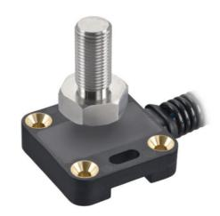
The NRH275DR is a no-contact, Rotary Position Sensor that is accommodated in a low profile (9.5mm) housing of compact footprint (36 x 35mm) with dual-redundant outputs. Versatile, factory programmable electronics, which are supplied from 5Vdc, can be easily set to one of two analog voltage output ranges or one of three PWM frequencies. In addition, the polarities of the analog outputs can be set to one of three combinations – both tracking in the same direction or one opposite to the other.
